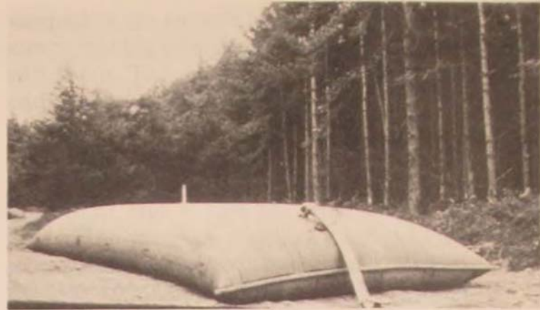
Figure 6(a). 12,500 gallon flexible tank
